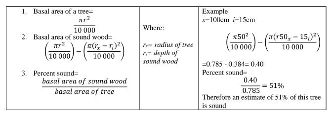
Figure 14. Calculating proportion of rot of the basal area of a tree
