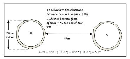
Figure 20. Measuring 50 metre distance between trees.
