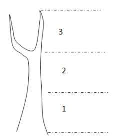
**Figure 13**. Division of a tree into 3rds for measuring broken tops
