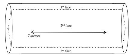
Figure 11. 'Face' of a monumental log is one-third of its circumference and the log length is minimum of 7 metres with one face that meets the defect allowances.
