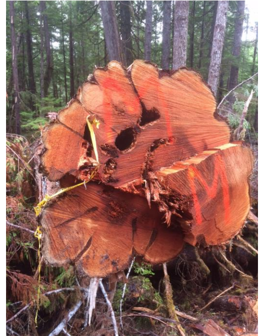
Photo 7. Butt of a tree with multiple bark seams. The highlighted example is from healing lobes that have joined. This example at the flare of the tree, would be considered an acceptable defect.
