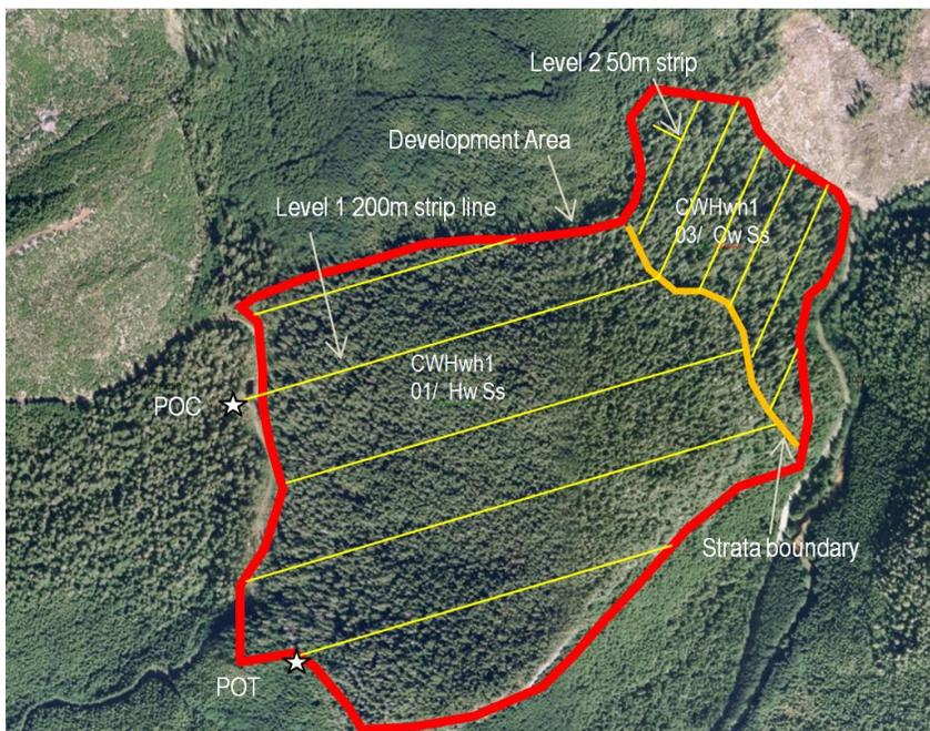
**Figure 5.** Block stratification example. In this case, the left or western most area, denoted by the 01 Site Series, is a Level 1 survey type and requires **less than** 100% block coverage. The right, or eastern most area, denoted by the 03 Site Series with a high concentration of Cultural Features, is a level 2 survey type and **requires 100%** block coverage.
